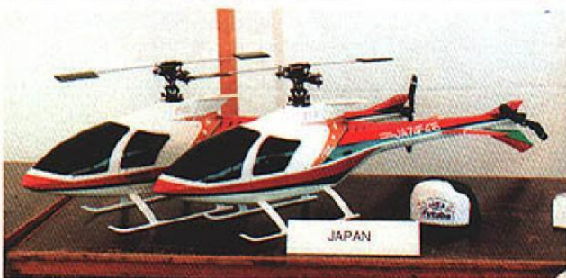
Left: Fifth-place F3C finisher Seiji Suwabe of Japan used Hirobo Eagle mechanics in modified Nova bodies. Right: The machines that captured the F3C World Championship for Japan's Kazuyuki Sensui: Kalt Omega mechanics in Aggressor bodies.
