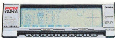
Large LCD readout screen displays plane selection and name, trim settings, exponential graphics, battery condition, servo reverse, mixing and more.
