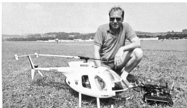
Gunter Knipprath (PEKA LUFTECHNIK) with his one bladed Hughes 500E. Notice that rotor head is flybarless. Counter weight is equal to blade and rotor blade holder, and balanced accordingly.
