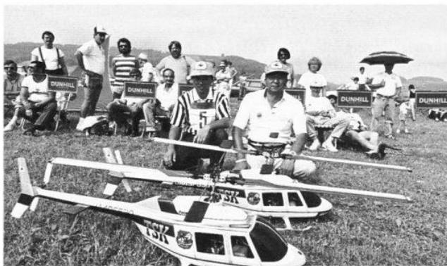
Tatsuya Iyobe with Shin Abe the Japanese team manager. Tatsuya's T.S.K. Jet Ranger used an Enya 60XF and Futaba 8SGHP radio.
