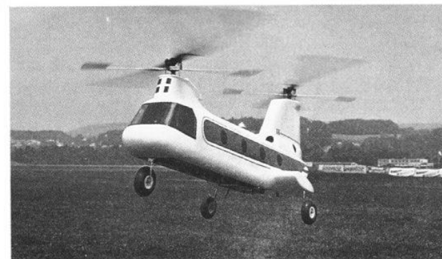
Another of Magnus Bisom's creations, a Vertol 107/CH46 using a 15cc Webra to drive both rotors.
