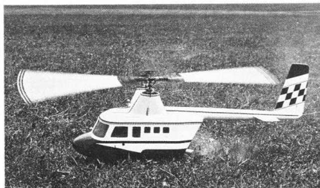
What's this? Flown in the demonstration by Magnus Bisom from W. Germany was this unusual 15cc Webra powered contrarotating main rotors 'Flettner'.
